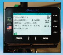
**In-cab computerized controller** for smart and easy precision application, monitoring and record keeping.
